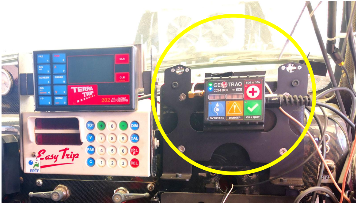
Installation of the Com-Box unit with bracket on the dashboard using bolts.
